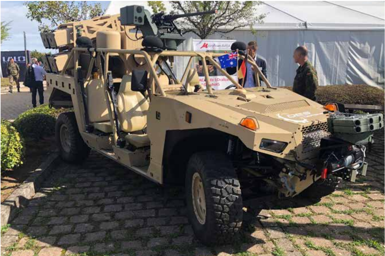
▲ Polaris DAGOR at the KSK Armaments Symposium 2022, here for four soldiers and with a launch container for guided missiles at the rear. (Photo: AF)
