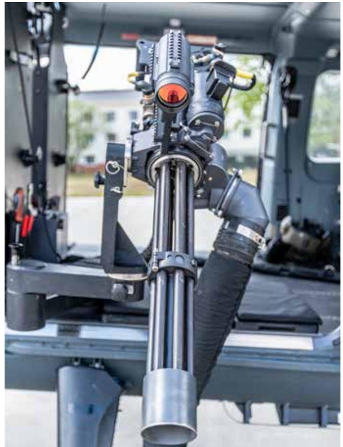
▲ The MG6, shown here on board an Airbus H145M LUH SOF. The weapon can be used on board of helicopters, the AGF SERVAL of the KSK or on tripods. Further platforms are now to be added. (Photo: Bundeswehr/Heyn)
