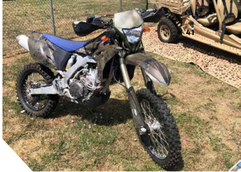
▲ Enduro from KSK based on the Yamaha WR450, tare weight <130 kg, max. total weight approx. 300 kg. (Photo: AF)
